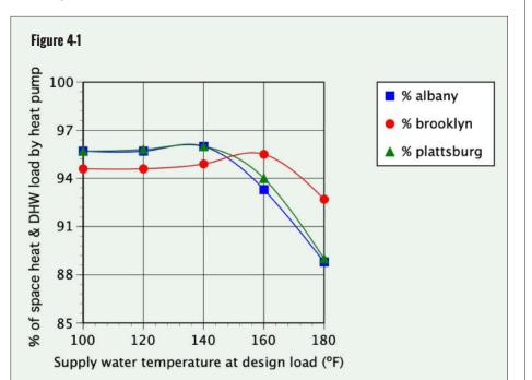
in Brooklyn, to just over 8,000 °F•days in Plattsburg. The air-towater heat pump modeled in the simulations had an enhanced vapor injection refrigeration system, and a nominal capacity of 4 tons. The simulation also included a yearround domestic water heating load of 60 gallons per day, heated from 50°F to 120°F.
