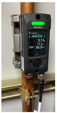
This meter can be quickly mounted to the outside of a pipe. It can be used with a wide range of pipe materials and sizes, as well as different fluids, and over a wide range of temperatures. Reported accuracy is +/-3% of the reading value. When equipped with optional platinum RTD temperature sensors, the meter shown in figure 3-8 can directly measure the  $\Delta T$ of a hydronic circuit and combine that measurement with flow rate to calculate the rate of heat transfer.
