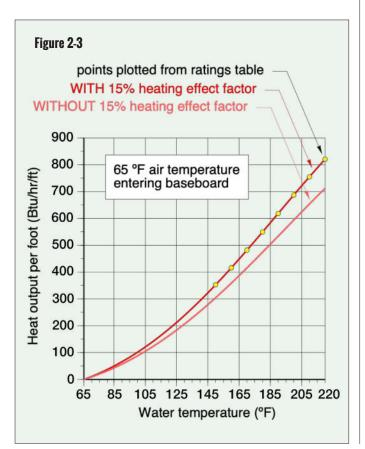
The lower curve is based on removing the 15 percent heating effect factor from the manufacturer's ratings.
