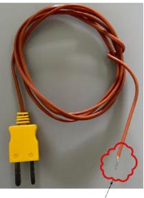
end of thermocouple — that senses temperature
