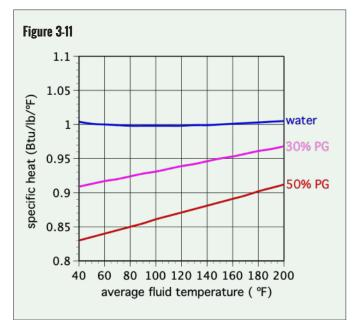
A dual temperature meter is used to measure the supply and return temperature of the circuit. The circuit's supply temperature is 120.6°F. The circuit's return temperature is 108.1°F. A strap-on ultrasonic flowmeter indicates a flow rate of 4.2 gpm. The system operates with a 30% solution of propylene glycol. Estimate the heat output of the circuit using formula 3-1.
