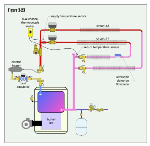
3. Turn on the test circulator and adjust its speed while monitoring the flow rate in the zone. Establish a flow rate approximately equal to the previously recorded flow rate for that zone.
