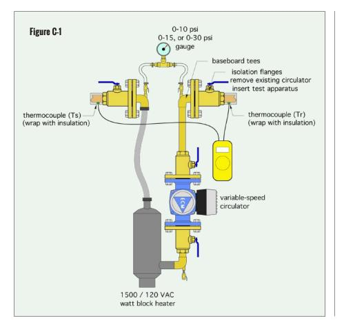
The test apparatus shown in figure C-1 was described in section 3. A procedure for using it to estimate the thermal performance of a circuit was also given.
