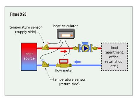
The two temperature sensors and the flowmeter provide information to a heat calculator that can determine the instantaneous rate of heat transfer and the total amount of heat that has passed from the heat source to the load over time.
