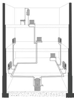
Today, a new hydronic system is likely to have a modulating/ condensing boiler or heat pump as its heat source and may only heat water to 110°F. Several components in the system, including the controls, the heat source, and the circulator(s), use microprocessor-based electronics to direct heat exactly where it's needed in a building, while optimizing fuel and distribution efficiency.
