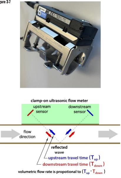
detected by the downstream sensor. The time between the pulse being emitted and detected in the direction of flow is very accurately measured.
