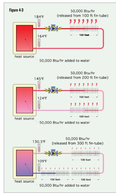
area separating the heating water from the room air will reduce the required supply temperature, while maintaining a given rate of heat output. This concept, along with representative numbers, is illustrated in figure 4-3.
