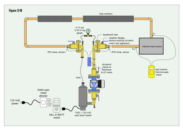
handle the full wattage at which the block heater can operate.
